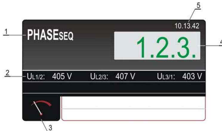
Figure 39: Display with PHASE SEQUENCE test result
