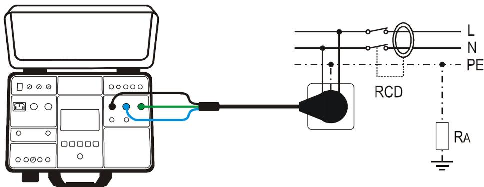
Figure 29: Connection of test cable to schuko socket
