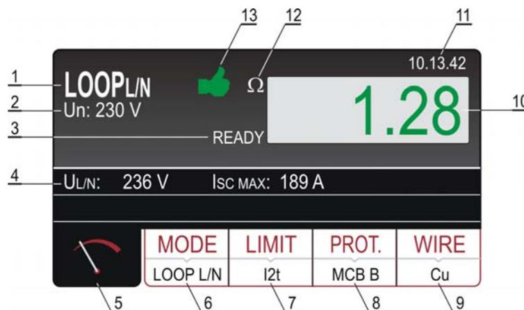
Figure 23: Display with LOOP L/N test result
