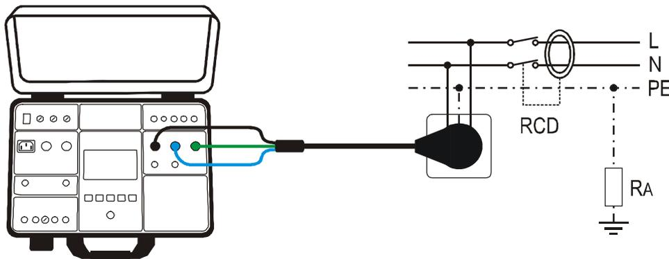
Figure 21: Connection of schuko test cable
