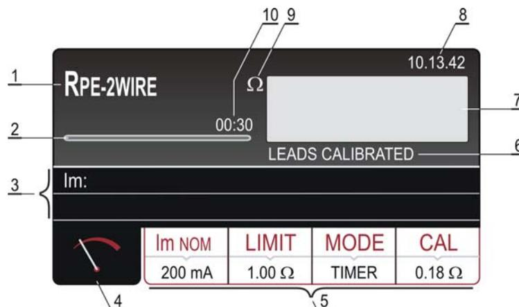
Figure 4: Basic measurement screen in RPE-2WIRE function
