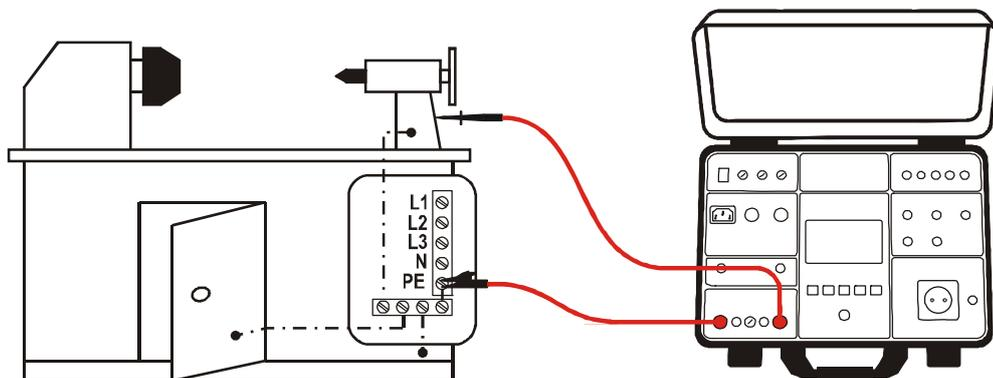
Figure 7: Connection of test leads in RPE-2WIRE function
