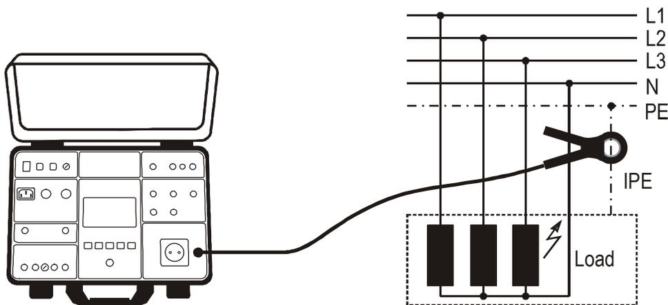
Figure 45: Connection of current clamp in I<sub>LEAK</sub> measurement, CLAMP mode
