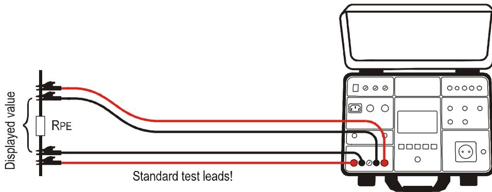
Figure 9: Connection of standard test leads
