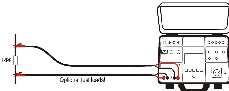
Figure 10: Connection of optional Kelvin test leads
