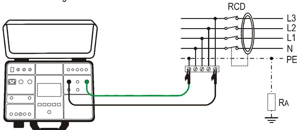
Figure 30: Connection of test leads to tested wiring
