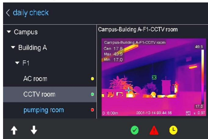
Figure 5-5 Check Inspection Result
