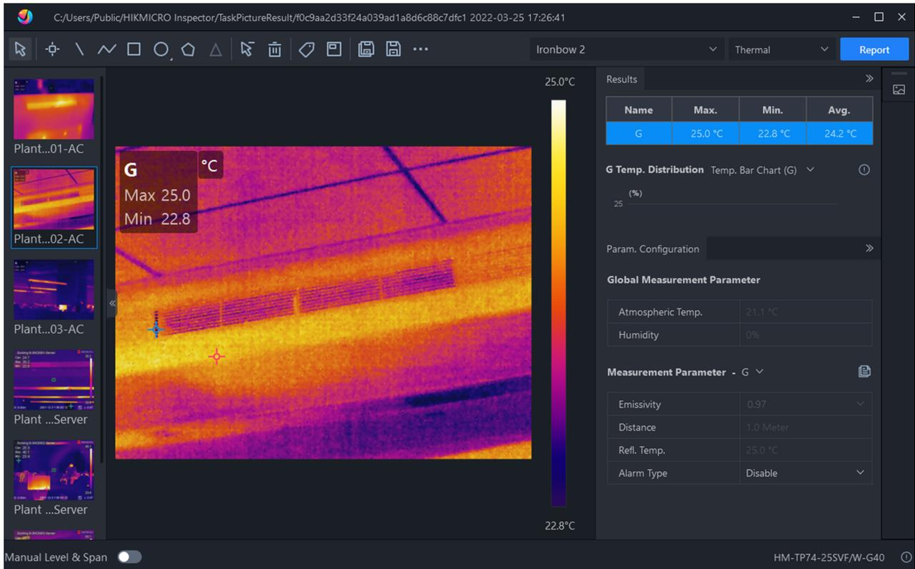
Figure 5-8 Analysis in HIKMICRO Analyzer
