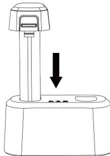
**Figure 2-2 Charge Battery**
