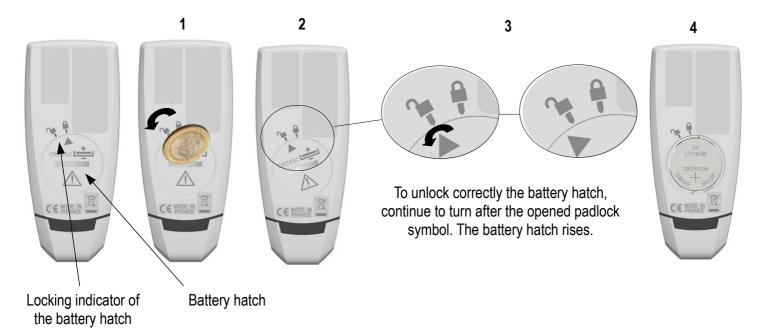
> Replace the battery hatch with the indicator in front of the opened padlock and close it by turning it towards the right in order to make correspond the indicator with the closed padlock.
