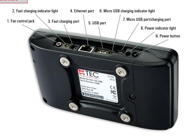
1. Fan control jack Input for a mono cable to connect the gauge to the fan speed controller.
