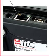
The Ethernet port on the gauge can be used to create a wired two-way communication link with a router or switch (the router or switch must be running DHCP Server).
