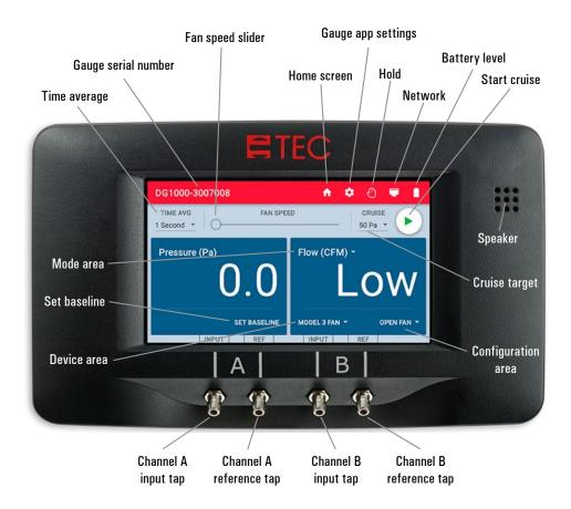
The function of Channel A is to measure a differential pressure between two locations. The Function of Channel B is to measure pressure at a device and convert it to an air flow.
