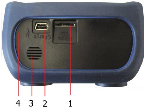
Fig. 2: Connection diagram (Interface side)
