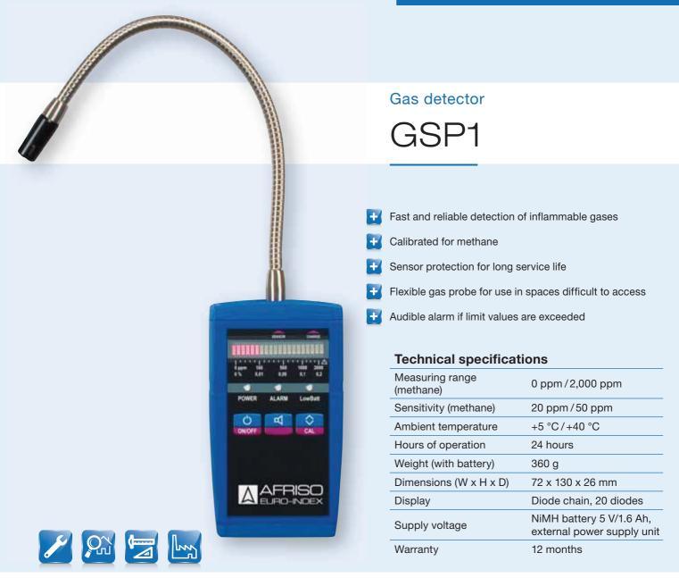
Application Detection of gas leaks in gas pipes as well as connection pieces and fittings, gas meters, gas burners and gas tanks (inflammable gases).
