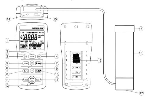
LCD Display: 4 digit display with a maximum of 9999 readings and the indicating signs of measured values, unit function symbols and decimal points etc. are displayed.
