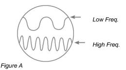
Since ultrasound is a high frequency, it is a short wave signal. Its' properties are different from audible or low frequency sounds. A low frequency sound requires less acoustic energy to travel the same distance as high frequency sound. (Fig. A)
