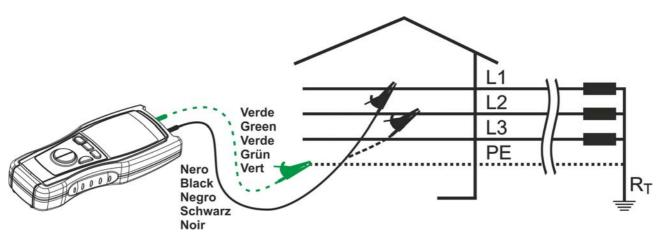
Fig. 7: Connection of the instrument's terminals during test
