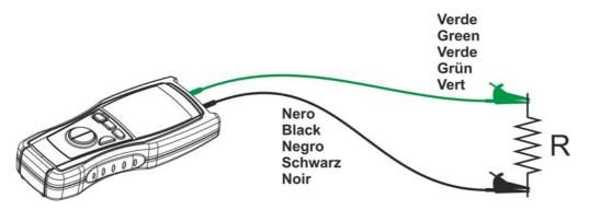
Fig. 5: Connection of the instrument's terminals
