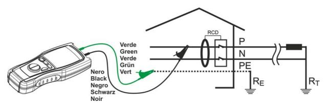
Fig. 14: Connection of the instrument's terminals during AUTO test
