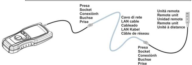
Fig. 8: Connections of the instrument's terminals during LAN tests
