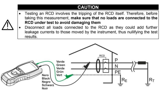
Fig. 12: Connection of the instrument's terminals during RCD test
