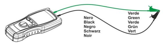
Fig. 10: Connection of the instrument's terminals during calibration procedure
