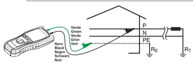
Fig. 3: Connection of the instrument's terminals during V  $\approx$  Hz test
