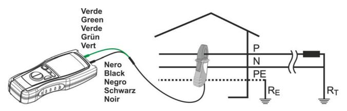
Fig. 4: Connection of the instrument's terminals during A = Hz test
