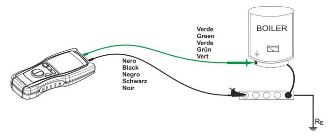
Fig. 9: Connection of the instrument's terminals during test
