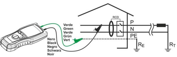
Fig. 11: Connection of the instrument's terminals during  $M\Omega$  test
