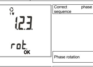
16. At the end of the test, if two cables belong to the same phase, the instrument emits a double sound to sigla the positive outcome of the test and displays a screen like this
