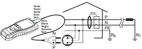
Fig. 13: Connection of the instrument's terminals during test
