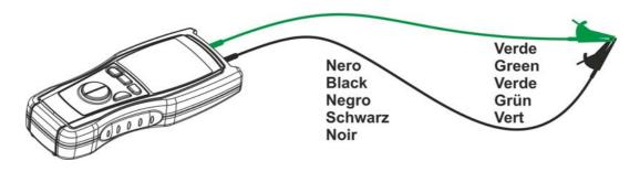
Fig. 6: Connection of the instrument's terminals during calibration procedure
