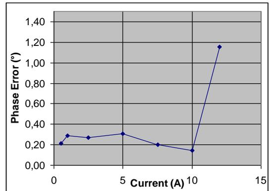
Figure 7: Phase error vs. current (for 5A range)
