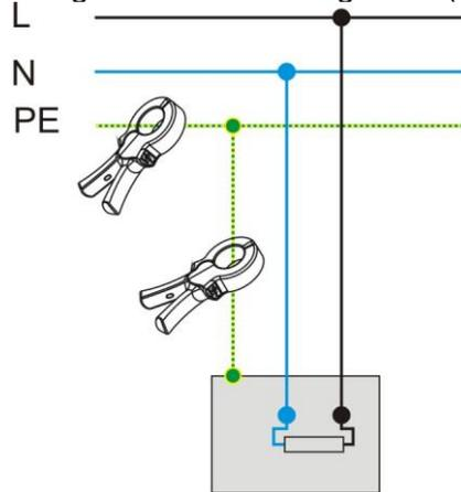
Figure 4: Leakage current measurement – direct method
