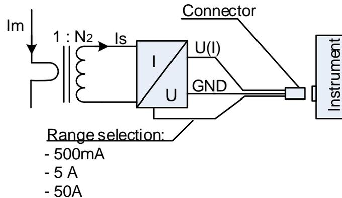
Figure 3: Current clamps A 1588 - block diagram
