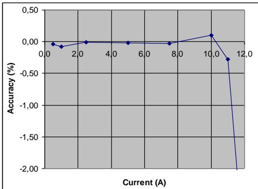
Figure 6: Accuracy vs. current (for 5A range)
