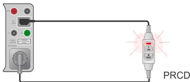
Figure 6.59: PE conductor (PRCD) test
