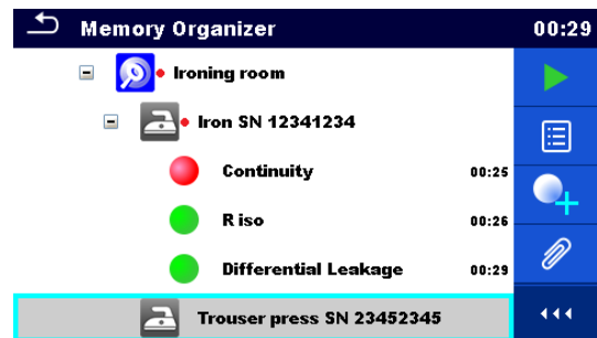
Figure 5.5: Status - Measurements completed with fail result(s)
