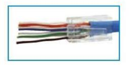
Step 4: Slide cable into connector until fully seated. Verify wiring order.
