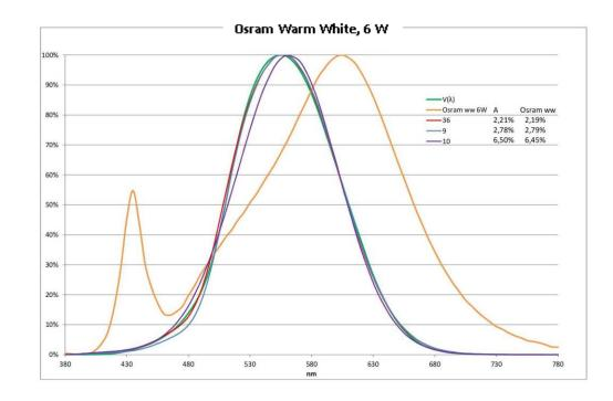
The OSRAM warm white 6 W is a typical white LED. It's based on the principle of a blue LED with a florescent coating.
