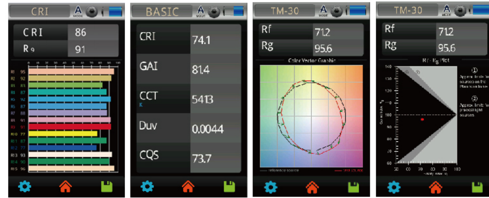
▲ Color Rendering Index(CRI/Ra) ▲ Gamut Area Index (GAI) Correlated Color Temperature (CCT) Delta uv (Duv) Color Quality Scale (CQS) ▲ TM-30-15 Color Vector Graphic
