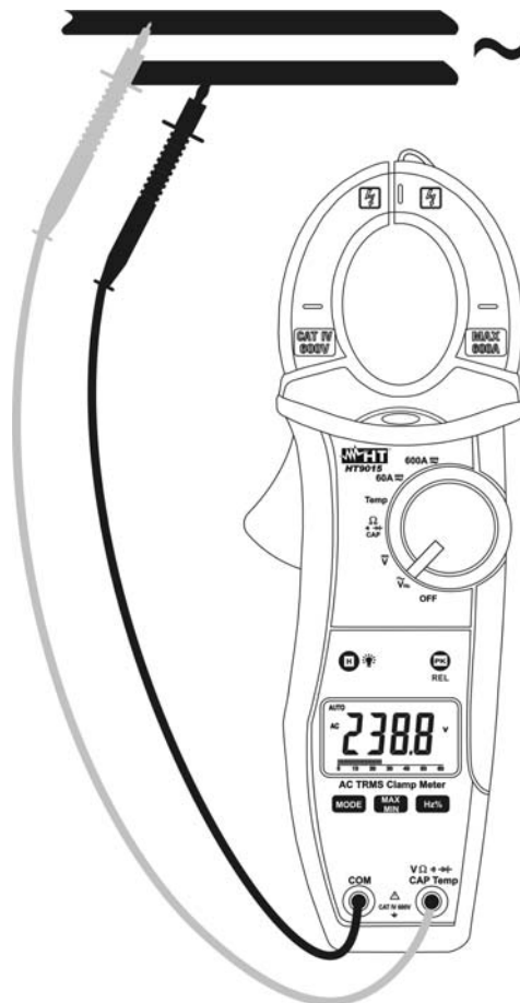
Fig. 7: Taking AC voltage measurements
