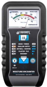
The Tramex Moisture Encounter 5 is a Dual-Depth, non-destructive moisture meter for instant moisture measurement and evaluation. Deep Depth penetration up to 30mm (1.25") & Shallow Depth penetration up to 10mm (0.40") 5 Ranges of sensitivity: Wood & Timber / Shallow Depth / Drywall & Roofing / Plaster & Tile / Masonry, making the Moisture Encounter ideal for testing in and through a wide range of materials in the building envelope.
