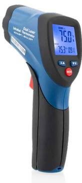
The IRT2 is a handheld, dual laser, non-contact Infrared Thermometer with 12:1 distance to spot ratio and audible and visible high/low set point alarms. It is used to measure and display surface temperatures within the range of -50°C to 650°C (-58°F to 1202°F) and has an accuracy of approximately 1 to 1.5% (see Specifications for details). The IRT2 has a fast response time (0.15 sec) and is powered with a 9V battery and complies with Class II UK/EU laser safety standard EN60285.
