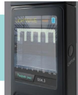
However, you may also see sharp cornered waves as we discussed earlier. As mentioned, these waves can sometimes be seen with LEDs with low quality drivers, registering higher flicker because of the sharp drop off in light intensity.
