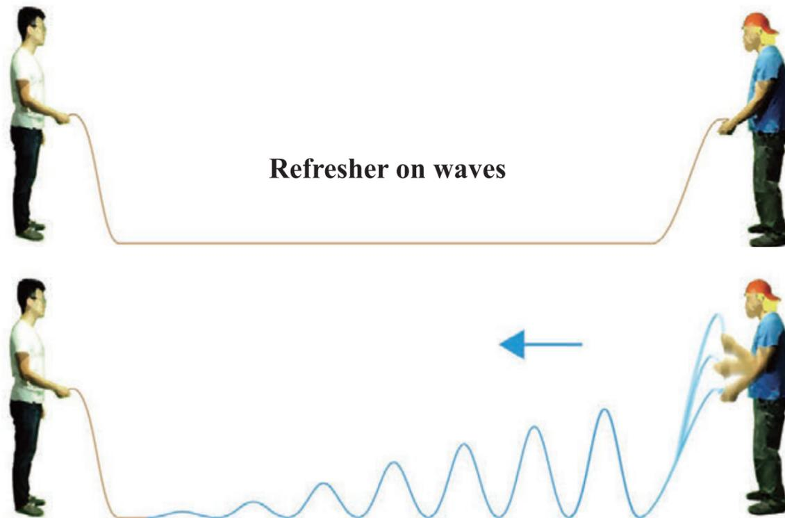
You can make a wave by jerking on the end of a rope. The wave traverses along the floor in a certain direction.
