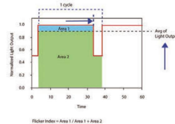
Some Dimmers and LED drivers do this purposely to reduce flicker, a method called Pulse Width Modulation or PWM, which we talked about earlier.
