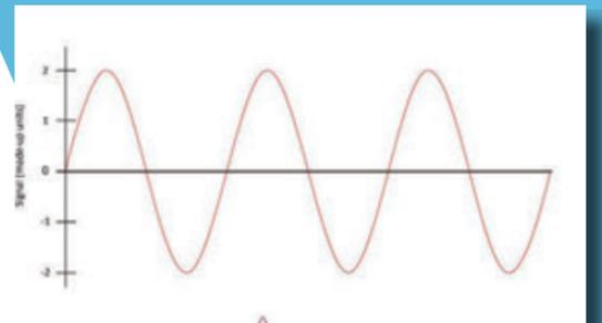
An oscilloscope connected to a home power mains can show a sine wave that reflects the alternating aspects of AC over time.
