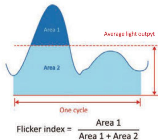
Let's start with an easier example (left) with square waves, whose areas are easier to comprehend (Area = L x W). Area 1 in the example represents the difference between the amount of high intensity light over low intensity light. Area 2 represents the residual amount of light shared by both high and low intensity light. To calculate the Flicker index would be Area 1 / Area 1 + Area 2. It's basically a percentage like Percent Flicker but you don't multiply by 100.
