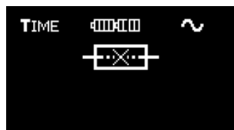
Fig. 3.2 The symbol of blown fuse
