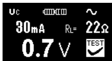
Fig. 3.10 Example of contact voltage measurement result
