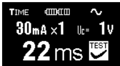
Fig. 3.12a Example of trip-out time measurement result
