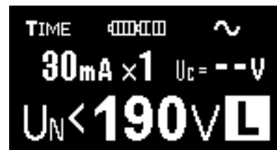
Fig. 3.16b Phase voltage present on the test tip
