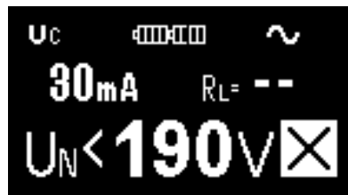
Fig. 3.8 Example of settings for contact voltage measurement
