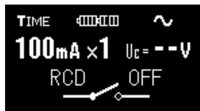
Fig. 3.5 Example of RCD trip-out during contact voltage measurement displaying
