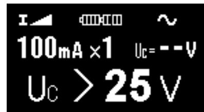
Fig. 3.4b Contact voltage > 25 V
