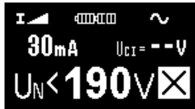
Fig. 3.14 Example of settings for trip-out current measurement
