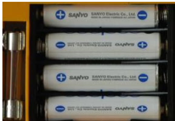
Fig. 4.1 Correct batteries/accumulators polarity and the fuse location
