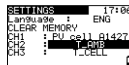
Figure 4-5: Use of temperature sensor selection
